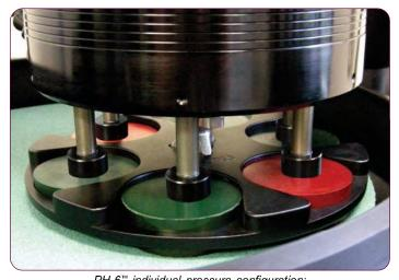
PH-6™ individual pressure configuration: six (6) individual pistons apply force to the mount(s) (2" mounts shown)
